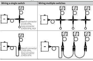
Maximum 30 unit of switches can be connected to a controller (SFC-N322)
